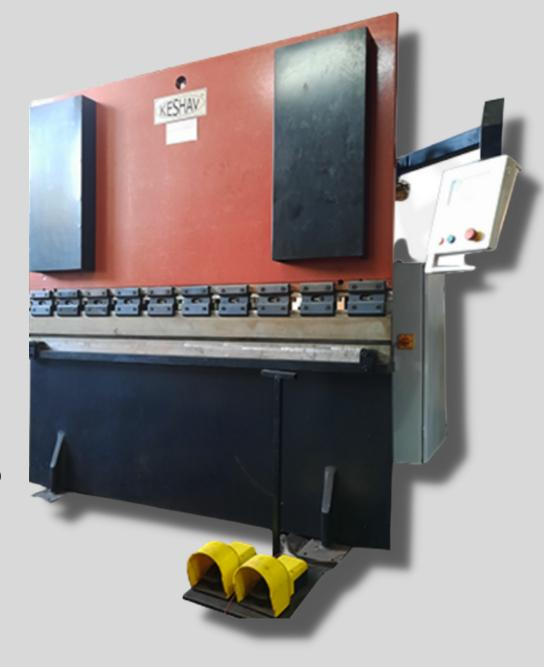
The program gives facility to bend different bending degree, different back gauge positions & different open positions. It has a facility to save different programs and same can be reloaded as & when required. The back gauge consists of Back Gauge Fingers, Ball Screw & Linear Bearing along with drive.
